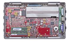
Inside the RUGGEDBOOK SR820s, the Samwelllabeled motherboard is extremely clean. It has fixed edge connectors on one side, and a separate I/O module on the other side. Having a discrete I/O module makes customization easy.
