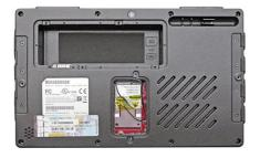
The battery compartment is protected by a flat metal plate secured with four Philips screws. The battery itself is a rectangular block. Its capacity is 38 watt-hours (7.4 Volts, 5,200mAh).
