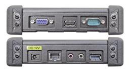
Samwell offers two different I/O configurations. One adds a standard DB-9 RS232 serial port, the other replaces that port with the window for the optional industrial-grade 1D/2D laser scanner. Our test unit included the following ports:
